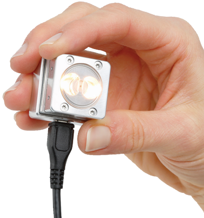
Figure 1. The NIRONE sensor weighs 15 g, and incorporates a MEMS Fabry-Pérot interferometer, an InGaAs photodetector, two tungsten lamps, and all of the control, processing, and communication electronics into one 2.5- × 2.5- × 1.75-cm box.
