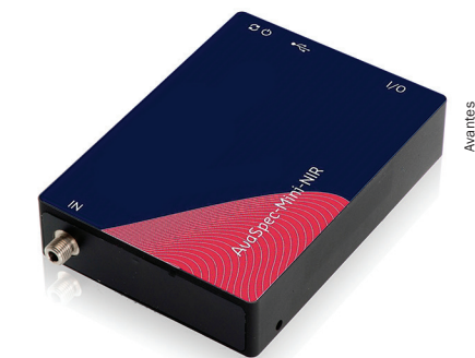
Figure 3. The AvaSpec-Mini-NIR symmetrical Czerny-Turner spectrometer.
