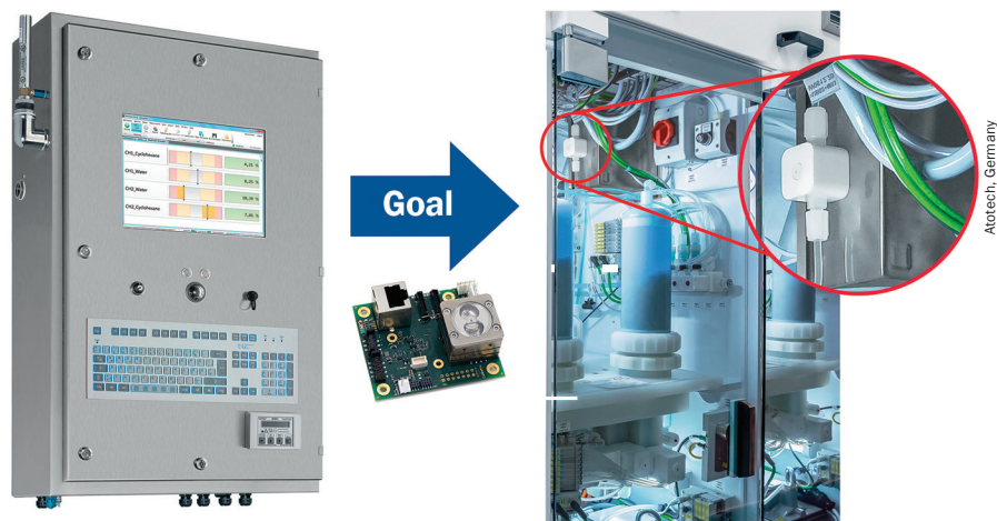
Figure 4. Cu and Fe online analysis, integrated in an electrochemical plating machine.
